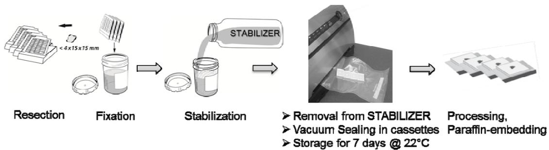
**Figure 1. Vacuum sealing in tissue cassette.** Rat tissue samples were fixed in tissue cassettes with the PAXgene Tissue FIX Container (50 ml). The fixative was replaced by PAXgene Tissue STABILIZER and tissue samples were vacuum sealed within the cassettes with a FoodSaver Vacuum sealer. After incubation in FoodSaver bags for 7 days at 22°C, the samples were processed and paraffin embedded.
