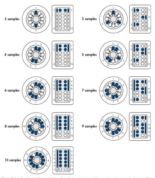
Figure 22. Loading the centrifuge and shaker. Centrifuge and shaker positions are shown for processing from two (2) to ten (10) samples. One (1) or 11 samples cannot be processed. The position numbers in the shaker rack correspond to the position numbers in the centrifuge. For processing twelve (12) samples, all centrifuge and shaker positions are loaded (image not shown).
