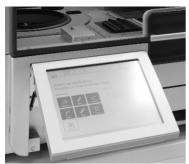
Figure 16. Pulled-out touchscreen of QIAcube Connect MDx.
