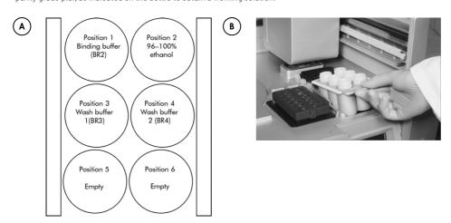
Figure 17. Loading the reagent bottle rack. [A] Schematic of positions and contents of bottles in the reagent bottle rack. [B] Loading the rack onto the QIAcube instruments (QIAcube shown as example).
