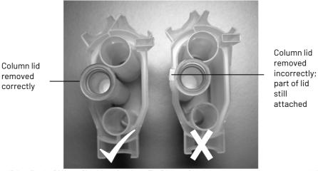
Figure 19. Loading the PAXgene Shredder spin column. The PAXgene Shredder spin column is loaded into the middle position of the rotor adapter. Cut off the lid before loading the column.
