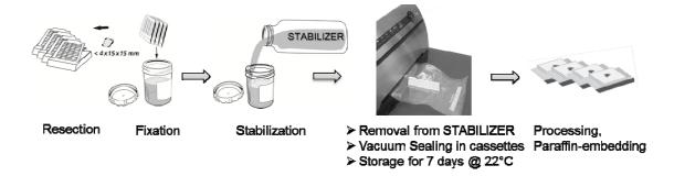
**Figure 1. Vacuum sealing in tissue cassette.** Rat tissue samples were fixed in tissue cassettes with the PAXgene Tissue FIX Container (50 ml). The fixative was replaced by PAXgene Tissue STABILIZER and tissue samples were vacuum sealed within the cassettes with a FoodSaver Vacuum sealer. After incubation in FoodSaver bags for 7 days at 22°C, the samples were processed and paraffin embedded.
