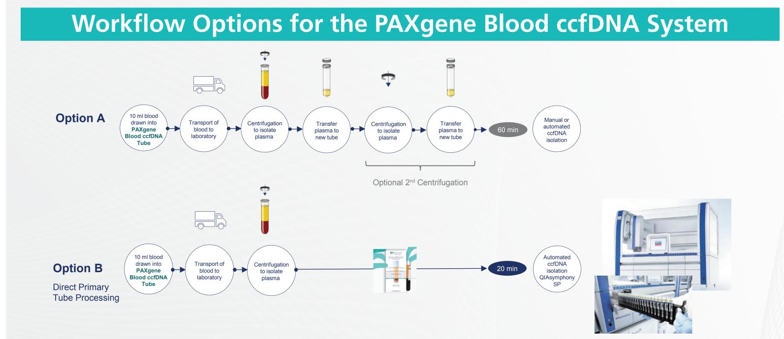
. Option A is the workflow described in the QIAsymphony PAXgene Blood ccfDNA Kit Handbook using the optional second centrifugation step. Option B is the new primary tube handling workflow using the PAXgene Blood ccfDNA Tube to be processed directly on the QIAsymphony SP instrument. Time savings based on processing a 24 sample batch.
